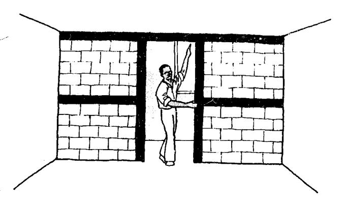
Interior walls should be built using columns and ring beams also, and they should be fastened securely to the outer walls. Doors should be placed in the center of the wall for maximum strength.
