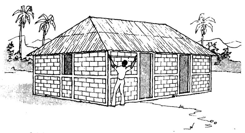
Each door or window should be a minimum of 36 inches from the corner. Doors and windows should also be separated by a distance of 36 inches.
