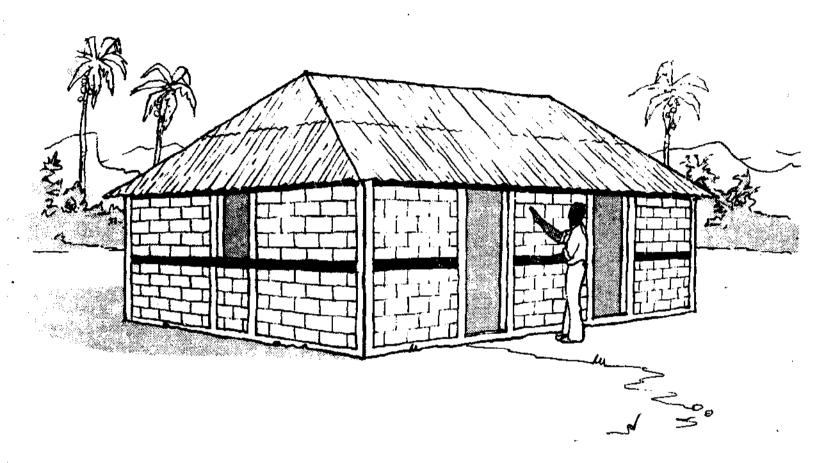
Build a reinforced concrete ring beam in the center of each wall.
