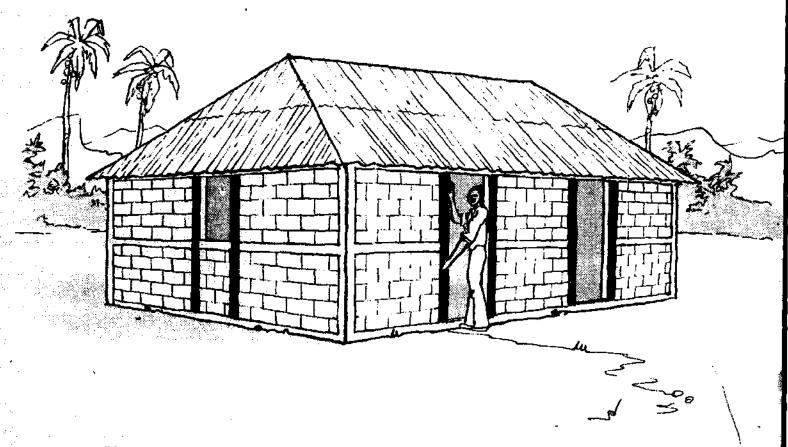
Place reinforced columns at the side of each door and window.
