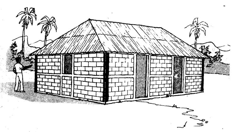
Place cement columns reinforced with iron rods in each corner.
