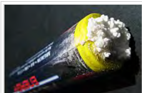
Potassium carbonate, formed from the hydroxide solution leaking from an alkaline battery
