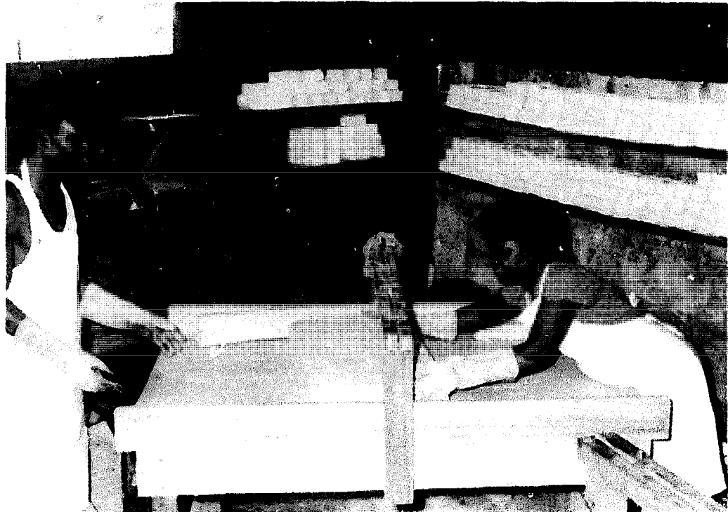
Plate 16: Soap cutting operation. The soap block is first cut into slabs before being cut into bars
