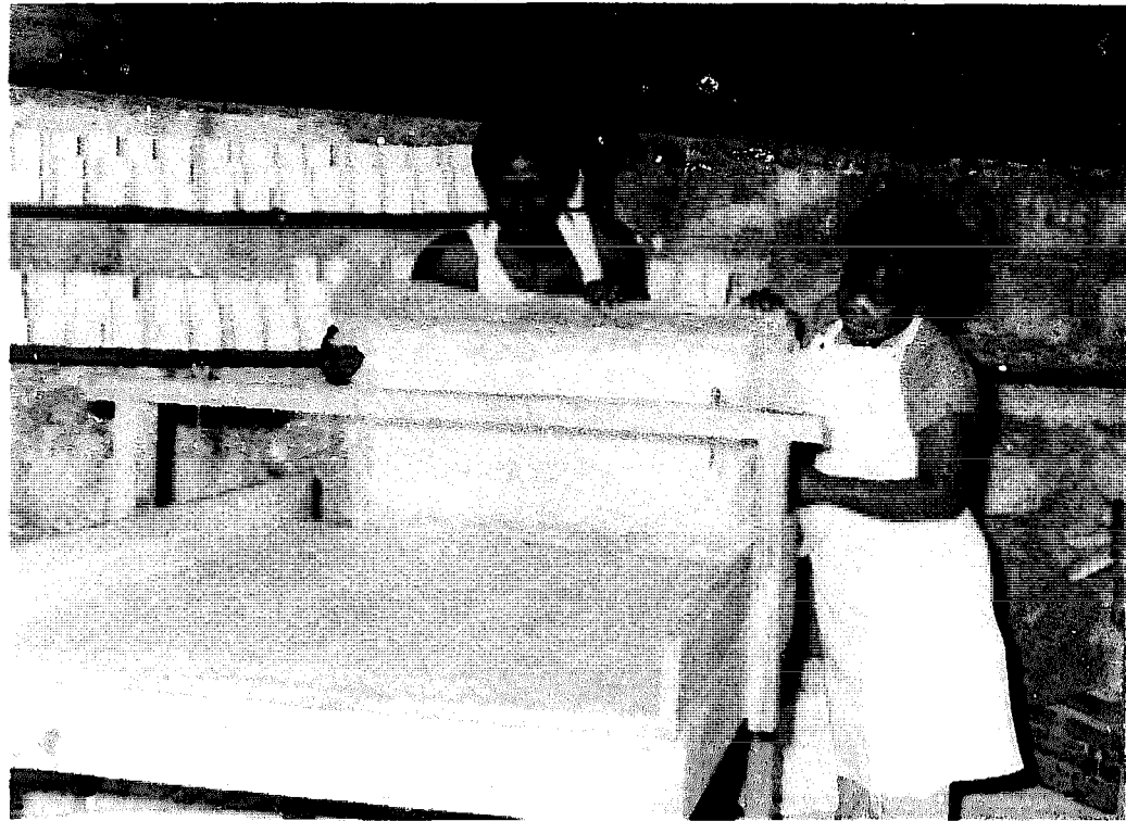
Plate 15: Removing soap from the soap moulding box for cutting
