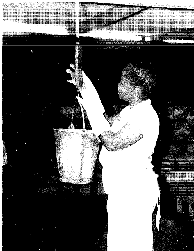
Plate 12: Weighing caustic soda with a spring balance
