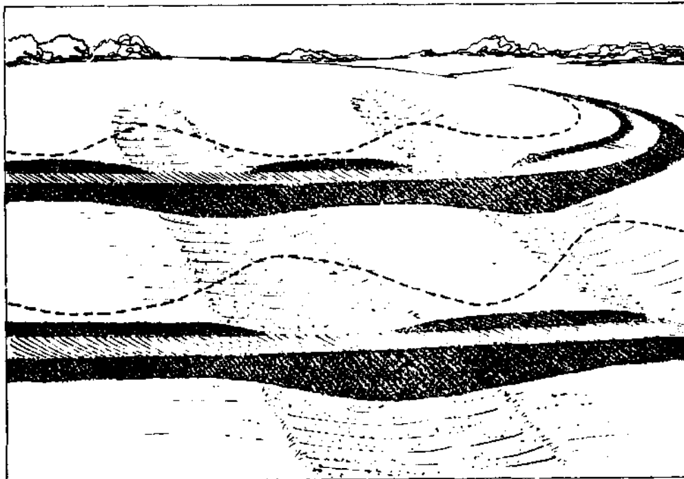
Fig. 9-24. Cut and fill parallel terraces. The dotted lines show where standard terraces would have been located.
