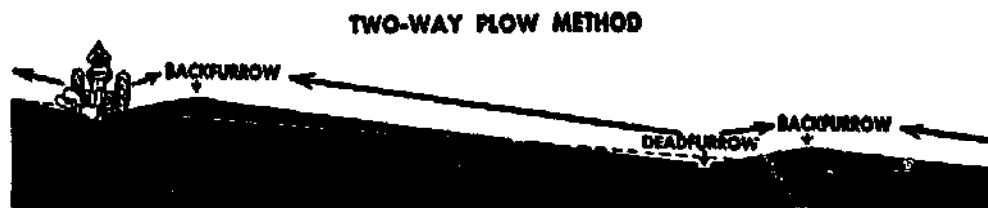
Fig. 9-10. Illustration showing the effect of plowing terraced land with the two-way plow. The arrows show the direction the soil is moved.
