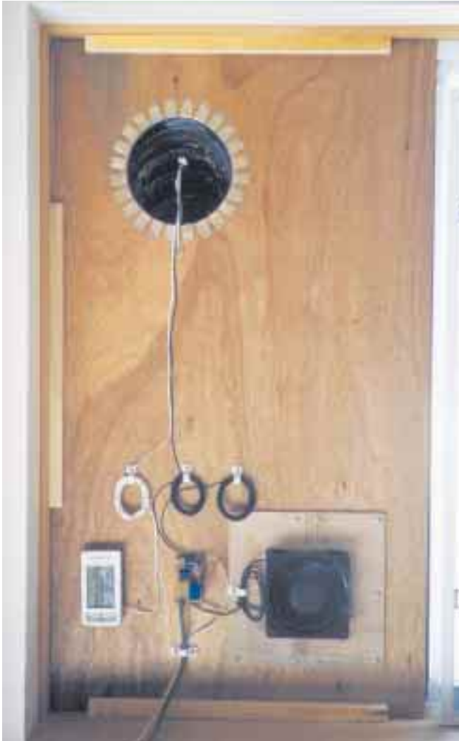
Insulated duct adapter panel, showing the fan in front of the cold air inlet (lower right), the hot air outlet (upper left), the temperature control circuit, and the dual thermometer.
