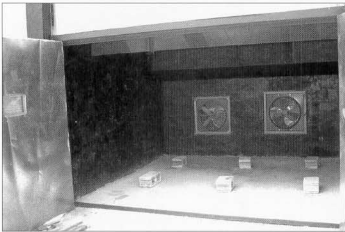
Figure 4 An open compartment of the solar kiln. The timber stack is placed on the blocks to allow air circulation below.
