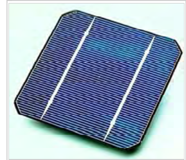
A conventional crystalline silicon solar cell (as of 2005). Electrical contacts made from busbars (the larger silver-colored strips) and fingers (the smaller ones) are printed on the silicon wafer.
