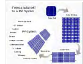
From a solar cell to a PV system. Diagram of the possible components of a photovoltaic system
