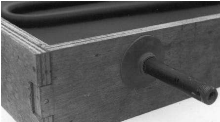
Slip rubber discs over the inlet and outlet pipe of the absorber.
