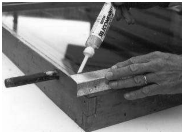
Fill-up the space between angles and glass-sheet with silicone-kit or putty.
