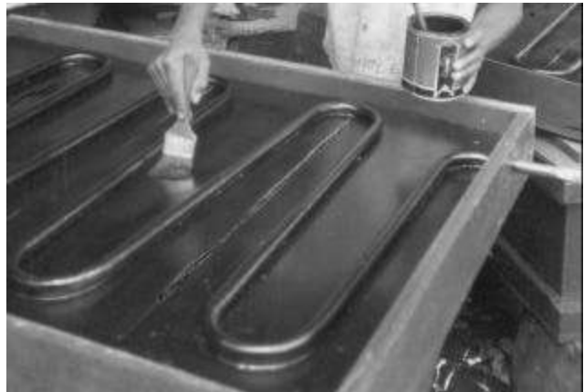
After the red lead paint or primer, paint the topside of the absorber with two layers of dull blackboard paint.
