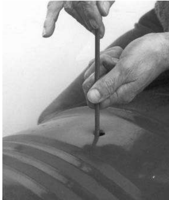
Photo 2: Debur the holes with a round file until the holes have diameter of 18 mm.
