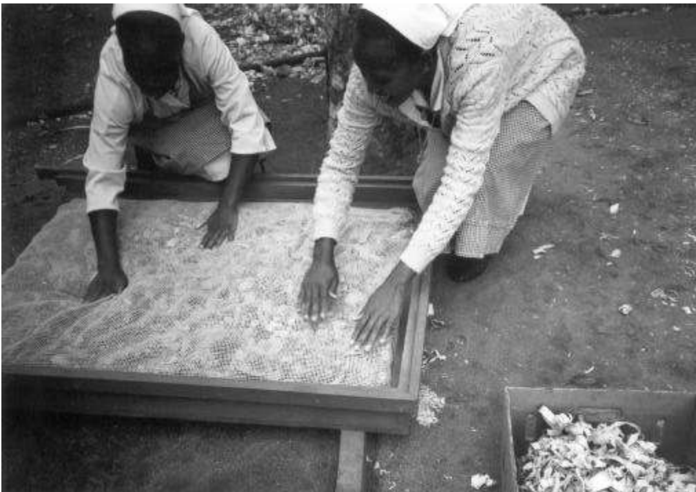
The insulation layer is put in the collector-box. The absorber is placed over the insulation layer next.
