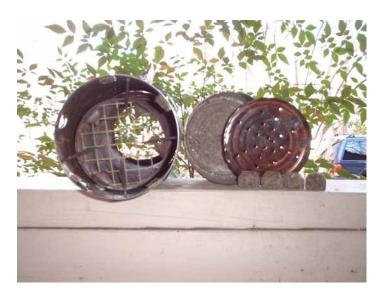
Looking from the bottom (top is unchanged), both bottoms have been cut out and ¼ inch hardware cloth has been shaped and inserted in the base of the burner. The church key tabs made from the can opener, on the cowling, have been bent down 180°. These rest on the rim of the ash holder (right), which provides a stable base for the stove.
