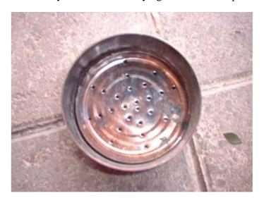
On top of the lug nuts I place the punctured bottom of the cowling I removed previously.
