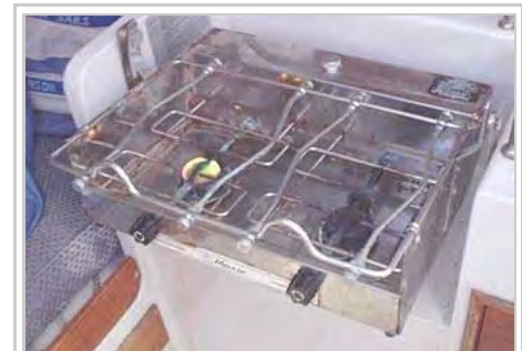
Two-burner spirit stove, with far burner on low heat
