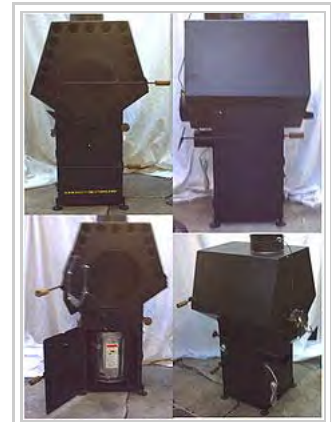
The pentagonal self-cleaning wood stove, is an EPA style secondary combustion air wood stove with a fan forced heat exchanger, thermostat, outside air intake with throttle, shakers, and ash drop for easy cleanup.
