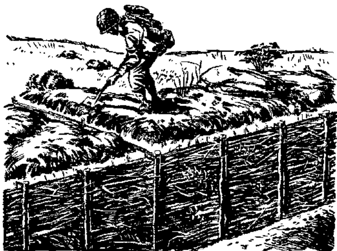
Figure 14. Continuous brush revetment.
