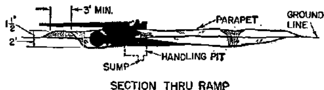
Figure 48. Emplacement for 155-mm gun M1. (Camouflage omitted.)
