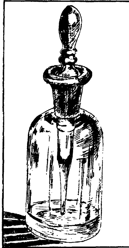
FIGURE 28. - Sketch of small bottle fitted with rubber-tipped pipette (as used for eyedrops) containing standard solution of phenol phthalein.
