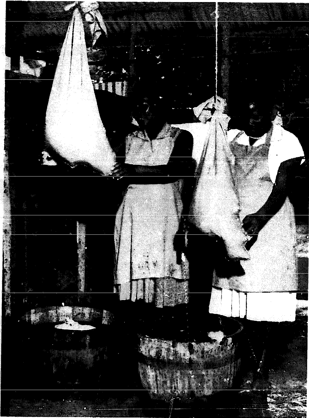
FIGURE 40. - Bag tanning of goatskins as practiced in village tannery in Africa. Courtesy Kenya Information Office, Nairobi
