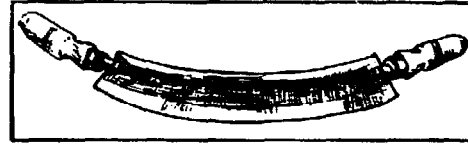
FIGURE 16. - Sketch of fleshing knife with two handles. One edge is concave and used for scraping; the other, convex, is very sharp and used for cutting.
