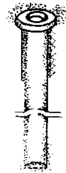
Bored Pit with Concrete Lining
