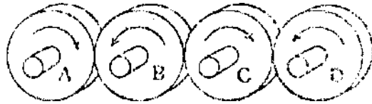
Fig. 2.—Train of gear wheels and relative motion of each wheel
