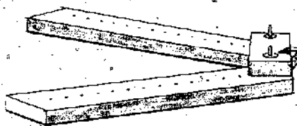
Use pieces of the same material to make two 2-inch by 5-inch swivel bars. Drill two 1/4-inch holes centered 1 inch from each end.
