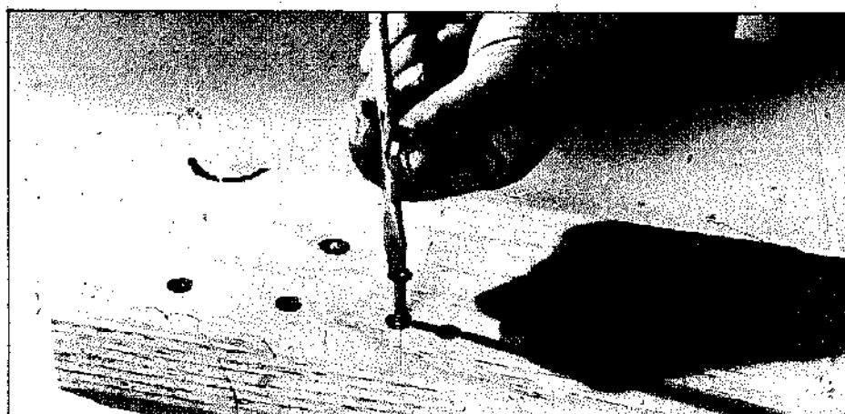
Once the screw is started, use your free hand as a guide to keep the driver in vertical alignment.
