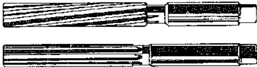
Figure 1-44.—Above—solid spiral flute reamer. Below—solid straight flute reamer.
