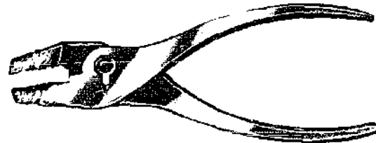
1.21.4B Figure 1-95.—Slipjoint combination pliers.
