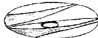
cut tool stock from discarded tractor plowdiscs
