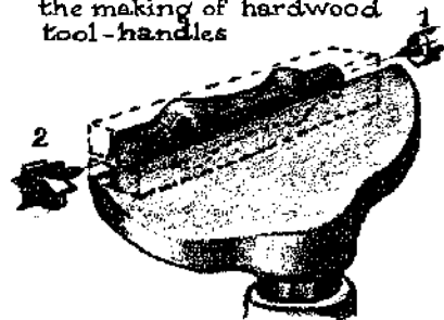
slant tool to cut nearest grain first
