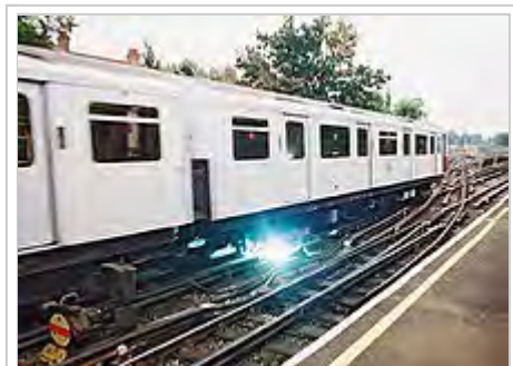
Electricity arcs between the power rail and electrical pickup "shoe" on a London Underground train
