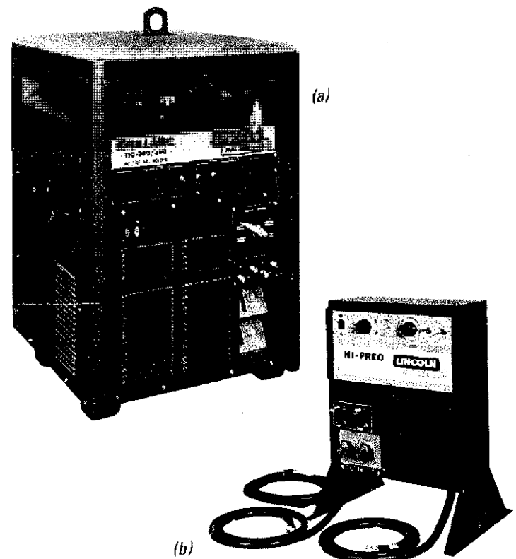
Fig. 4-29. (a) A transformer-rectifier welder designed for AC-DC TIG welding or for AC-DC welding with consumable covered electrodes; (b) a high-frequency generator for adapting an AC or DC metal-arc welder for use with the TIG process.
