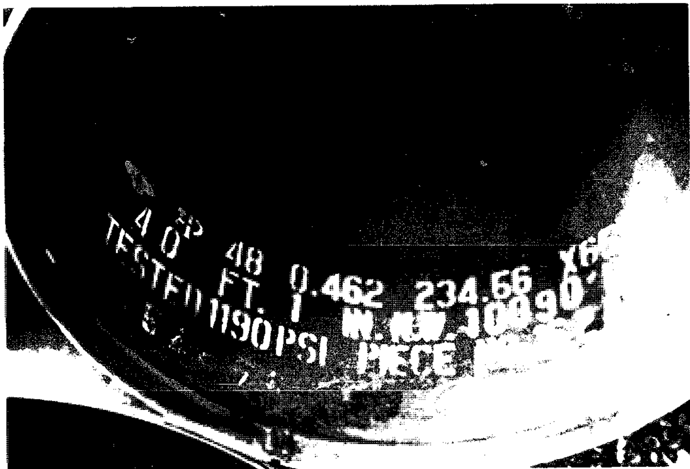
Close-up of the above pipe showing the end protector. Pipe is manufactured to API specification X65 (vanadium treated), 48-in. diameter, 0.462-in. wall thickness, 40 ft. 1 in. long, net weight 10,090 lb., tested at 1,190 psi.
