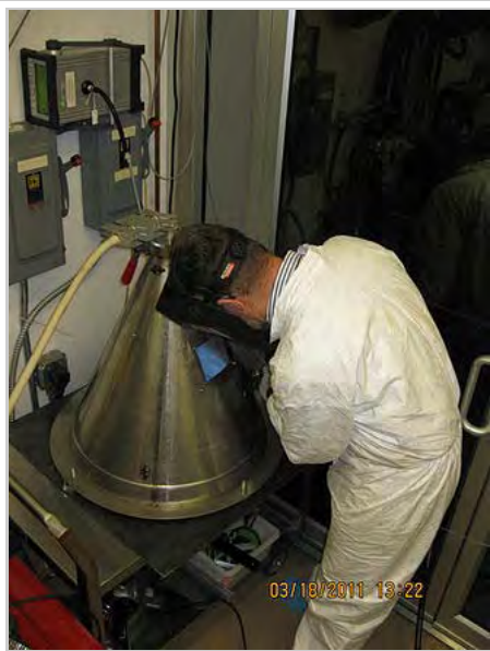
A chamber designed to contain welding fumes for analysis
