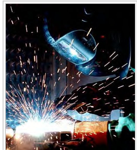
Gas metal arc welding (MIG welding)
