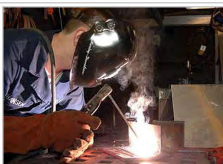
Shielded metal arc welding
