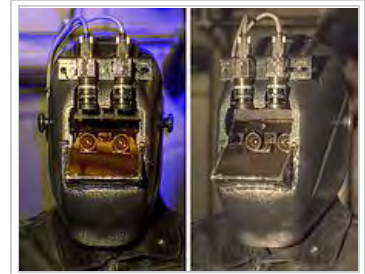
MannGlas welding helmet. Unlike Speedglas, the MannGlas helmet implements high-dynamic-range imaging (HDR) to augment the image in dark areas and diminish it in bright areas, thus implementing Computer-mediated reality.
