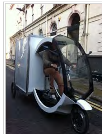
A modern electric cargo trike in use in London, with a payload of up to 250kg
