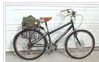
A bike equipped with an after market electric hub motor conversion kit, with the battery pack placed on the rear carrier rack
