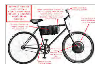
Diagram illustrating a standard bicycle converted to an e-bike using a retail conversion kit
