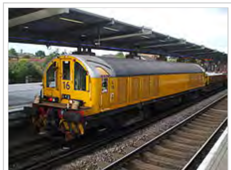
A London Underground battery-electric locomotive at West Ham station used for hauling engineers' trains
