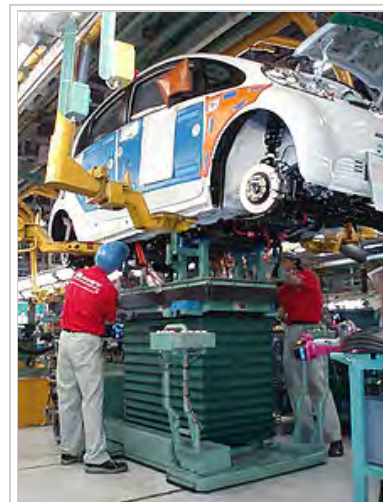
A Mitsubishi i-MiEV having its batteries installed
