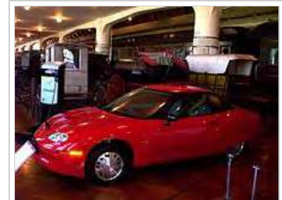
The General Motors EV1 had a range of 75 to 150 miles (240 km) with NiMH batteries in 1999.
