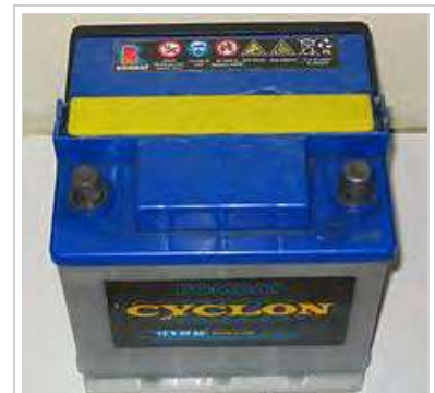
Old: Banks of conventional lead-acid car batteries are still commonly used for EV propulsion
