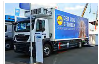
Electric truck e-Force One. Battery pack between the axles.
