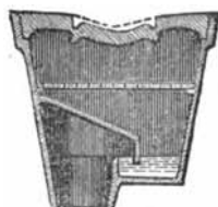
Fig. 163.—Section of a Stable Trap with a Fixed Syphon and Tray.
