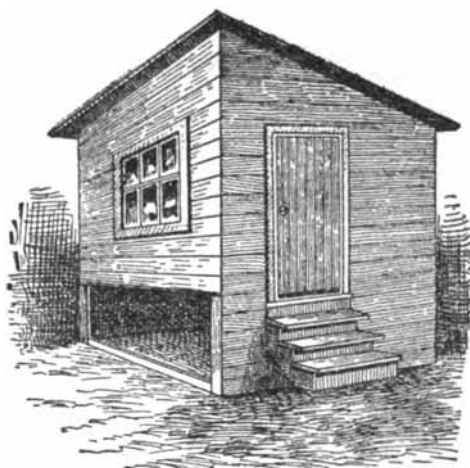
Fig. 10—Scratching Room Under Poultry House
