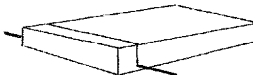
FIGURE 2. WHEN THE SOAP IS FIRM, REMOVE IT FROM THE MOLD AND, USING A THIN WIRE OR KNIFE, CUT IT INTO BARS.
