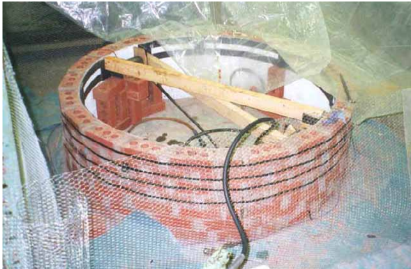
Figure 10 – Specimen under test, showing expansion ring
