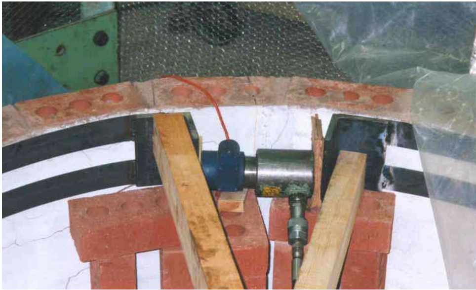
Figure 11 – Specimen under test, showing close up of hydraulic jack and load cell
