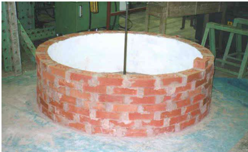
Figure 4 – Brick masonry cylinder specimen
