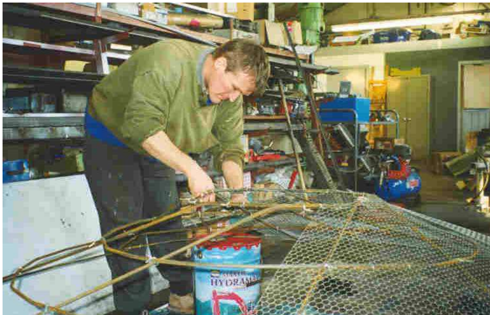
Figure 10. Applying the chicken mesh.
