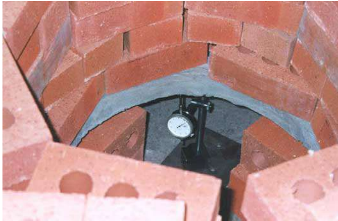
Figure 3 – dial gauge in place to test deflection of cover under load
