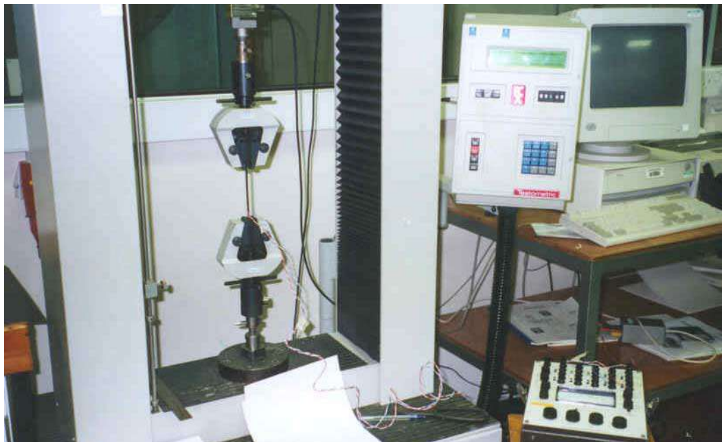
Figure 6 – Calibration of strain gauges using tensometer
