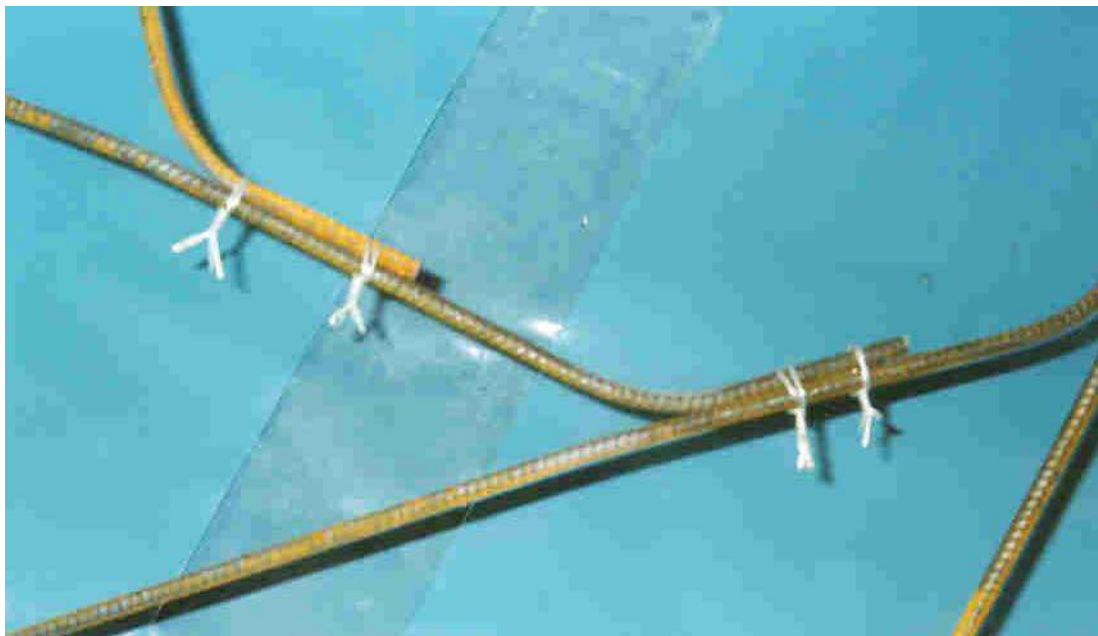
Figure 6. Arrangement for tying spokes to each other.
