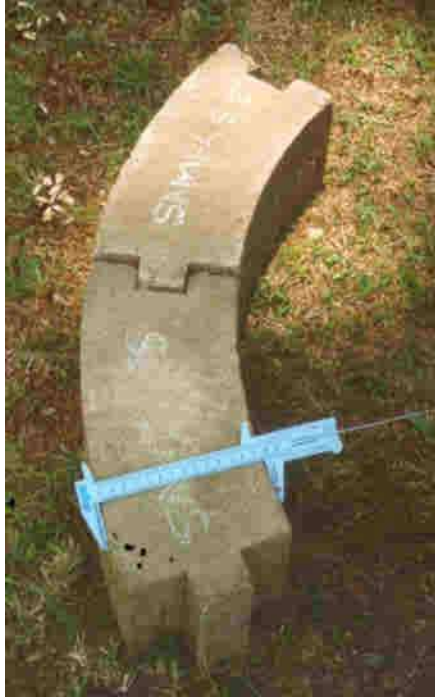
Figure 11 – Showing the interlocking blocks used for the tanks
