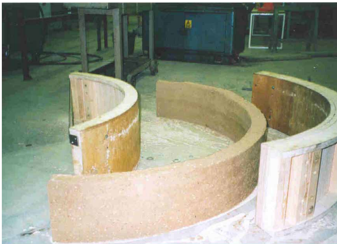
Figure 5 – A section of wall rammed between the wooden shuttering shown after removal of the shuttering
