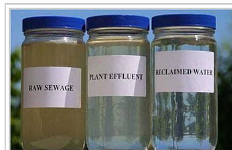
Samples of different types of (waste)water, starting with raw sewage then plant effluent and finally reclaimed water (after several treatment steps)
