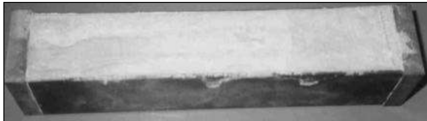
Figure 5.15 Micro crack development in restrained sample
