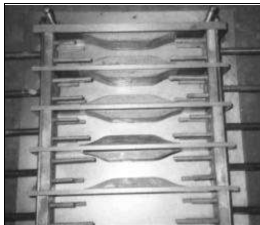
Fig. 5.3 moulds used to cast samples
