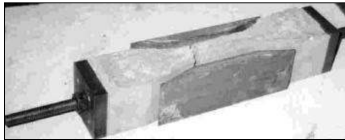
Fig 5.7 Wooden inserts used to neck samples
