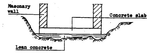
II. Non-reinforced concrete: To make foundations, floors
