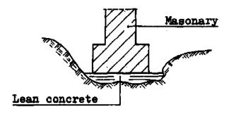
2. Example: Foundation of a spring collection chamber.
