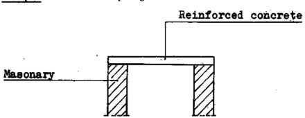
Note: The decision to use reinforced or non-reinforced concrete is a matter for the engineer, and it should be shown on the site drawings.
