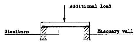
Due to dead load and additional loads such as people, earthfill, snow etc. the slab will get tensile stresses at the bottom. So in this place we must put some steel-bars into the concrete.
