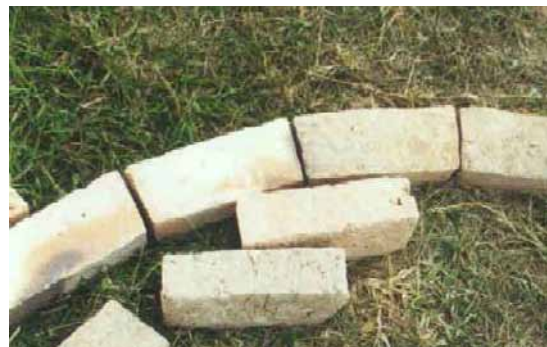
Figure 7b - The bricks with profiled ends
