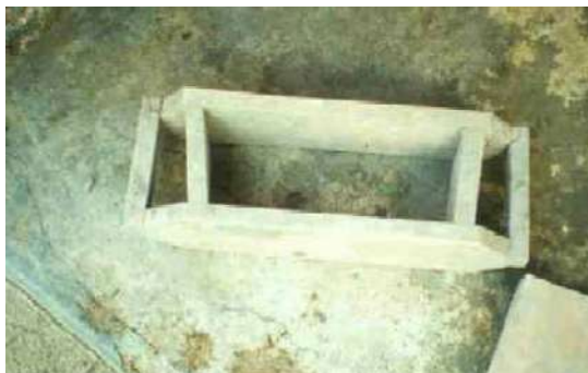
Figure 7a – Showing the mould used for casting the bricks used for the parapet wall
