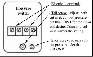
its rate of rise (this indicates flow rate). Does it rise to a certain point and then slow way down, long before it shuts off? If so, your system needs a pressure adjustment.
