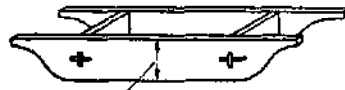
6" High for sand 12" High for gravel 2' 6" X 2' 6" BOTTOMLESS BOX FOR GAUGING CONCRETING AGGREGATE
