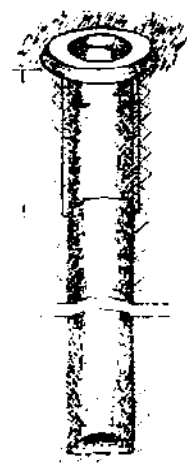
Bored pit with concrete lining
