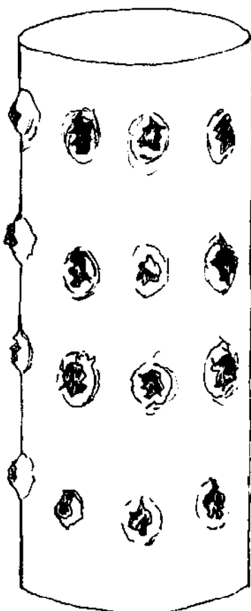
FIG. 15-5. PUNCTURED METAL CASING USED AS WELL SCREEN
