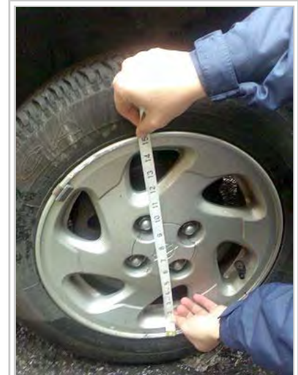
Measuring an outside rim diameter to approximate wheel size
