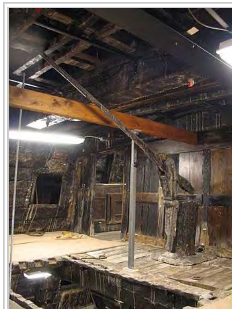
The still-intact aft bilge pump of the Swedish 17th century warship Vasa as seen from the upper gun deck.
