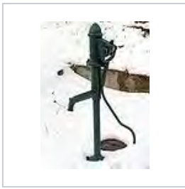
Hand-operated, reciprocating, positive displacement, water pump in Košice-Ľahanovce, Slovakia (walking beam pump).
