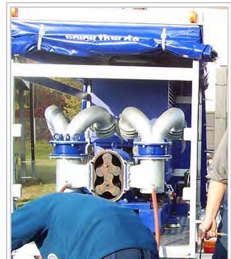
Lobe pump (5m 3 /min or 1886 barrel/h) of THW
