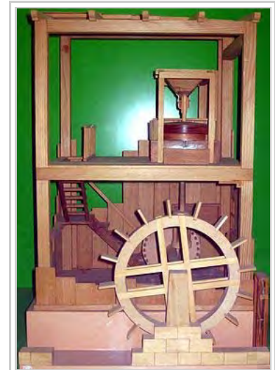
Model of a Roman type Roman water-powered grain-mill described by Vitruvius. The millstone (upper floor) is powered by an undershot waterwheel by the way of a gear mechanism (lower floor)
