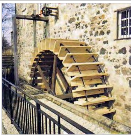
A breastshot waterwheel at Dalgarven Mill, United Kingdom
