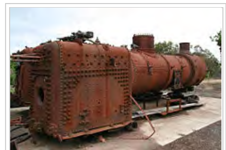
1950s design steam locomotive boiler, from a Victorian Railways J class
