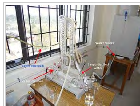
Typical laboratory distillation unit
