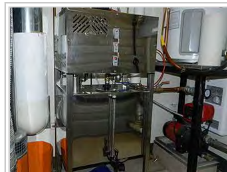
A boiling water distiller. Boiling tank on top and holding tank on the bottom.
