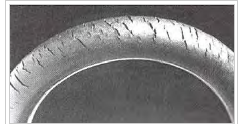
Ozone cracking in natural rubber tubing
