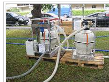
Portable water purification unit used by International Red Cross and Red Crescent.
