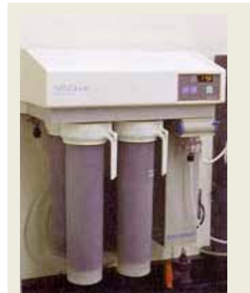
Laboratory grade water deionizer system that uses four mix bed resins, and activated carbon and particle filters.
