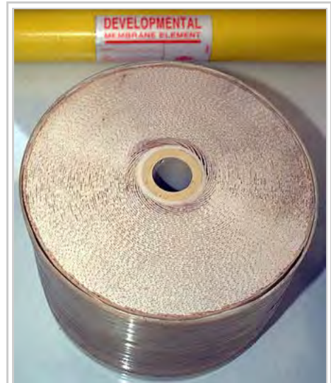
A semipermeable membrane coil used in desalination
