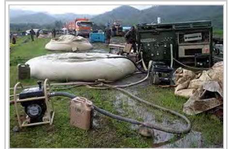
United States Marines from Combat Logistics Battalion 31 operate reverse osmosis water purification units for relief efforts after the 2006 Southern Leyte mudslide
