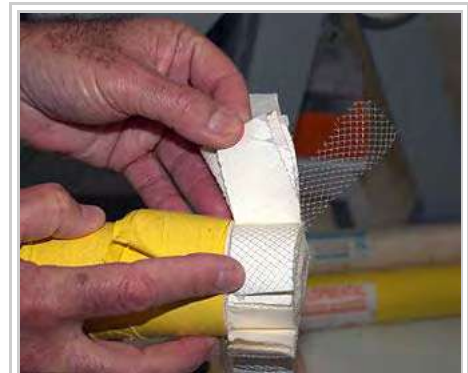
The layers of a membrane
