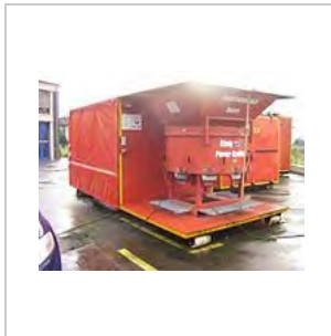
A German, roller container mounted, sandbag filling machine
